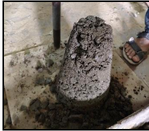
Fig. 3. Process of slump cone test of waste glass powder concrete"
