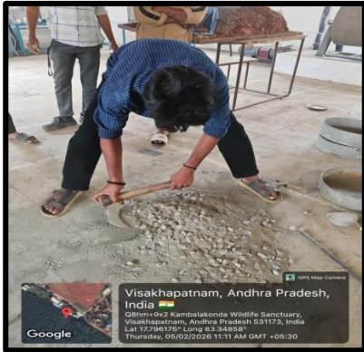
Fig :4 dry mixing
