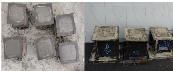
FIG.3.4. A.2 CUBE CASTING
