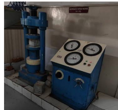
FIG 4.1.2 COMPRESSIVE TESTING MACHINE
