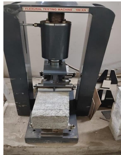
FIG 4.2.1 FLEXURAL TESTING MACHINE
