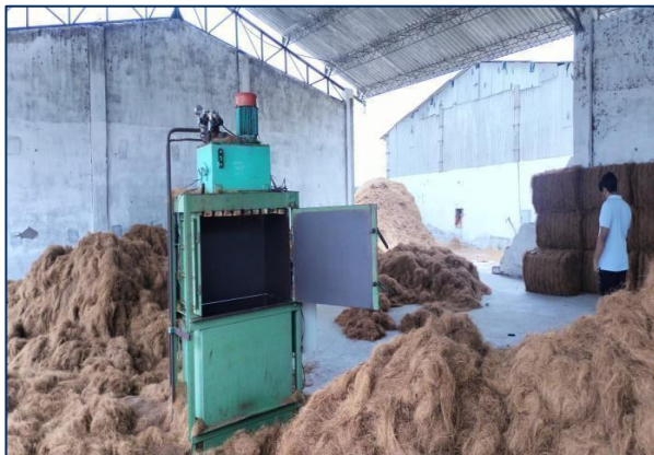
Fig 4.11: Hydraulic compressing of the first-grade fiber
