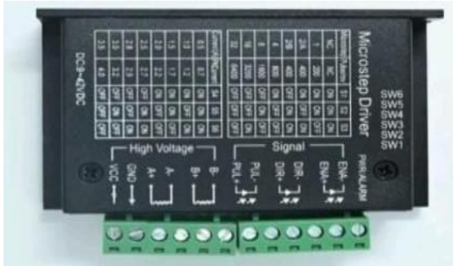
Figure8: Micro step driver
