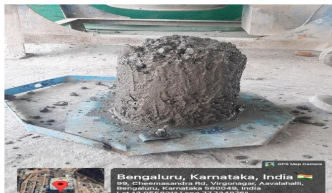
Fig -1: Slump sample
