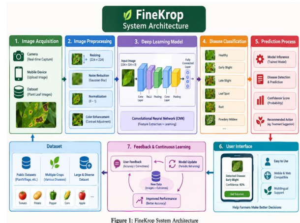
Figure 1: FineKrop System Architecture
