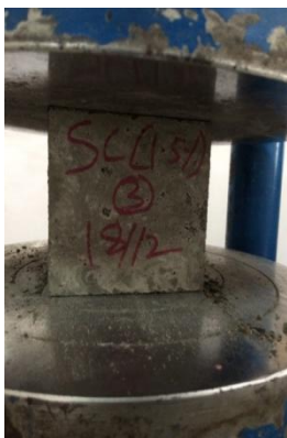
Fig -3 compressive strength test
