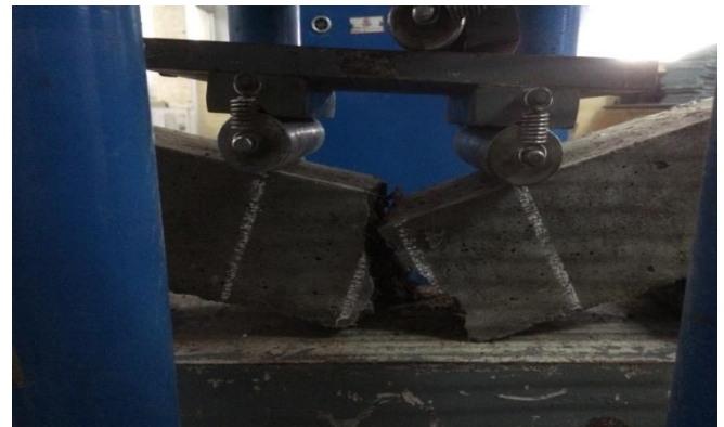
Fig -5 Flexural strength test
