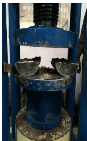
Fig -4 Split tensile strength test
