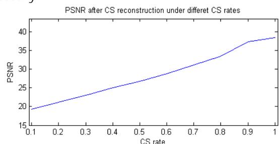
Figure.3CS reconstruction distortion when AC coefficients are transformed to the CS domain.
