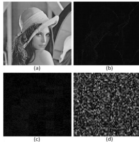
Figure.2(a)Original image; (b)Image in 8×8 DCT domain; (c)DCT coefficient after CS transformation; (d)Image reconstruction with the wrong CS matrix. (CS rate 1.0 is chosen here, similar effects are observed under other CS rates).
