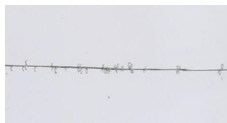
Fig-4: Pure water with 100 ppm Triton X-100 at Heat flux = 61.53 Kw/m 2
