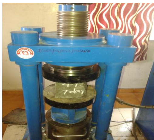
FIGURE 1: COMPRESSIVE STRENGTH TEST SETUP
