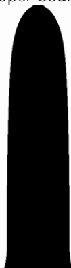
Fig-4: NAND SIMP solution to centrally loaded column problem on a 750 x 750 mesh and V_{frac} = 0.2
