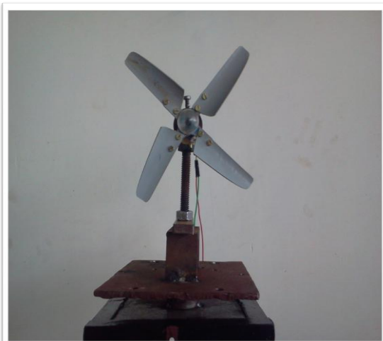
Fig -3.2: Experimental setup of bare wind turbine
