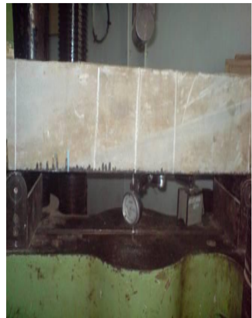
Fig.3 Beams test set up
