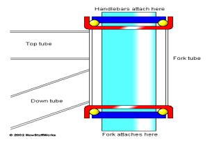
Fig -11: Fork Tube Attachments [11]
