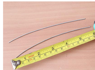
Fig 3: Strip of Platinum Coated Nickel Wire
