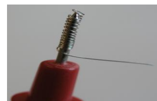
Fig 4: Winding of Platinum Wire
