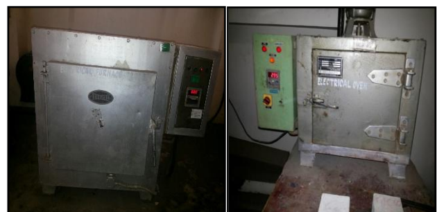
Fig-4 Specimen kept in Furnace and oven at 600°C and 300°C
