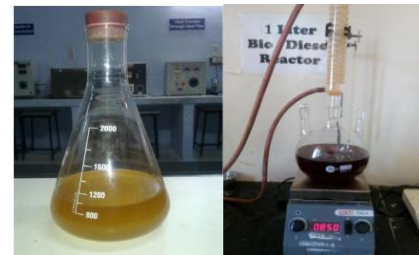
Fig -2.2: Transestrification Process of Mahua oil
