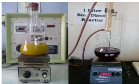
Fig -2.1: Esterification Process of Mahua oil
