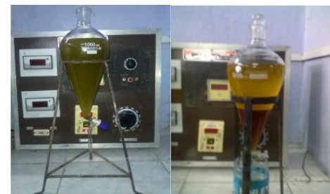
Fig- 2.3: Settling Process
