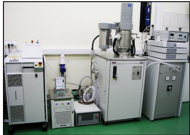
Fig -3: NETZSCH LFA 427 equipment Co-efficient of thermal expansion:
