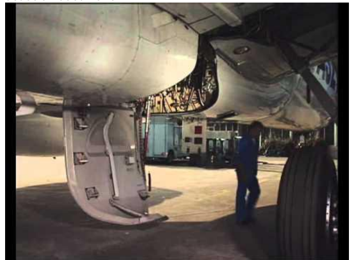
Fig -1: Main landing gear door panel of A320
