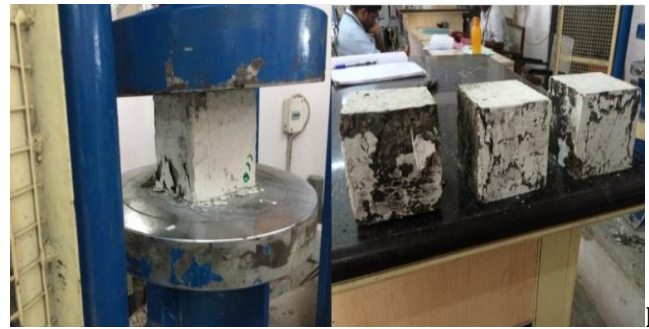
Fig -3 Cube specimen under test
