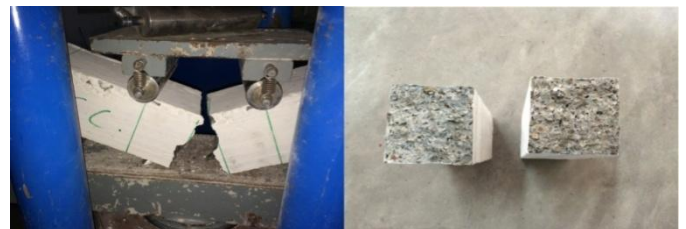
Fig -4 Flexural beam specimen under test
