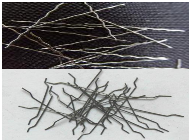
Fig -1: crimped and hooked steel fibres
