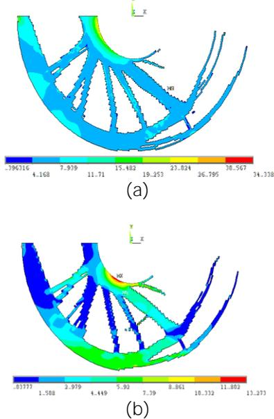
Fig.1.9 Von mises stress induced in structure for (a) Isotropic (b) Orthotropic
