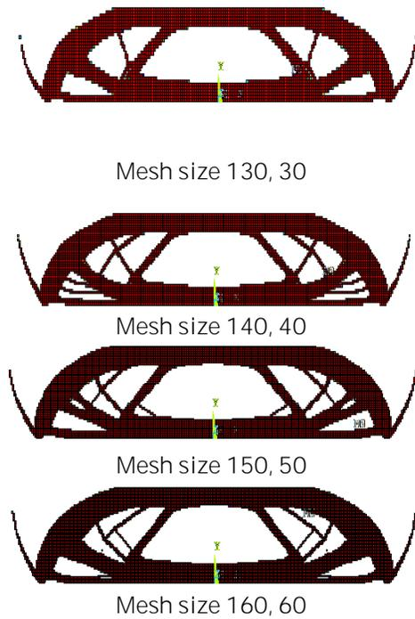
Fig. 3.3 Optimal topologies for different mesh densities for Orthotropic material Model 5 ( $V_0 = 50\%$ )
