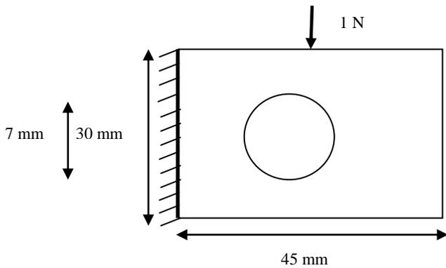
Fig.2.6 Geometry and boundary condition of overhanging beam
