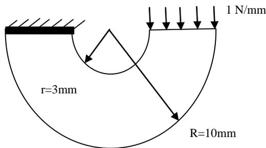
Fig.1.6 Geometry and boundary condition of overhanging beam
