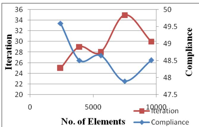
Fig. 3.4 Effect of number of elements on compliance and iterations for Orthotropic material Model 5
