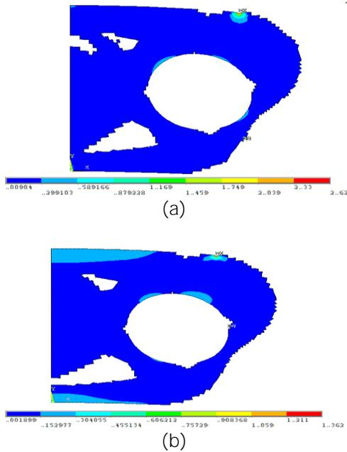
Fig. 2.9. Von misses stress induced in structure for (a) isotropic (b) orthotropic
