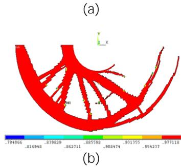
Fig. 1.7 Optimized shape for (a) Isotropic material (b) Orthotropic material
