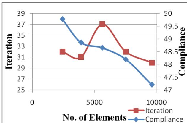
Fig. 3.2 Effect of number of elements on compliance and iterations for Isotropic material Model 5
