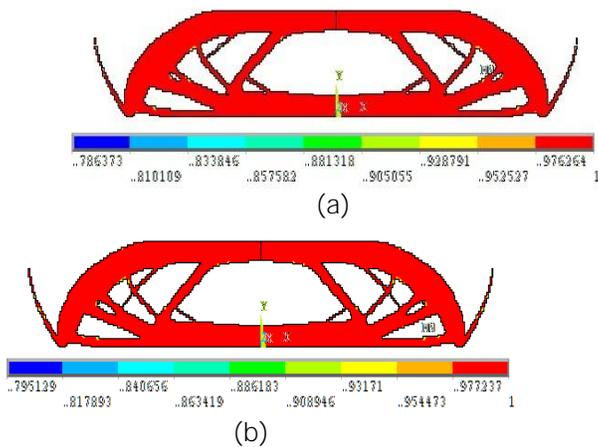
Fig. 1.2 Optimized shape for (a) Isotropic material (b) Orthotropic material
