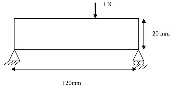
Fig.2.1 Geometry and boundary condition of overhanging beam
