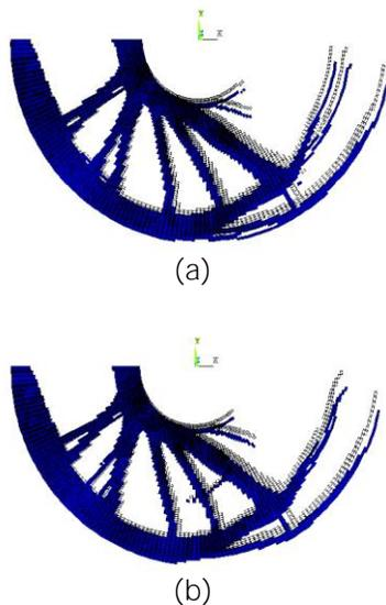
Fig. 2 Deformed and un-deformed shape obtained for (a) Isotropic (b) Orthotropic
