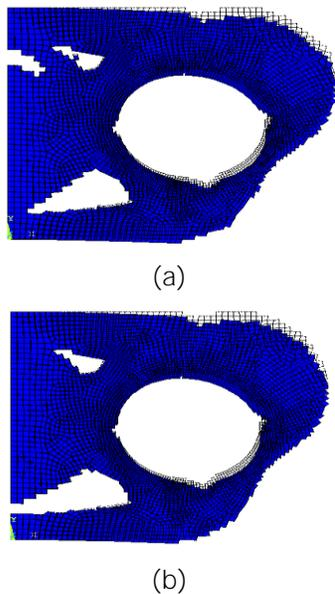
Fig. 3 Deformed and un-deformed shape obtained for (a) isotropic (b) orthotropic
