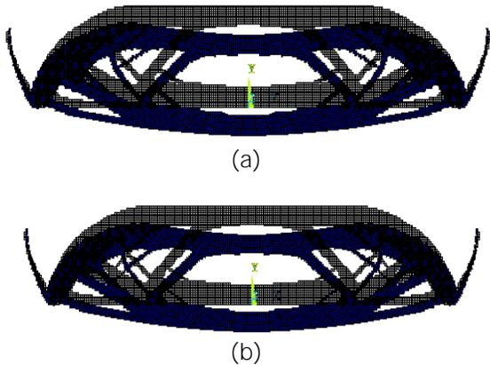
Fig. 1.5 Deformed and un-deformed shape obtained for (a) Isotropic (b) Orthotropic
