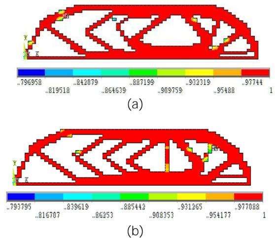
Fig. 2.2 Optimized shape for (a) Isotropic material (b) Orthotropic material
