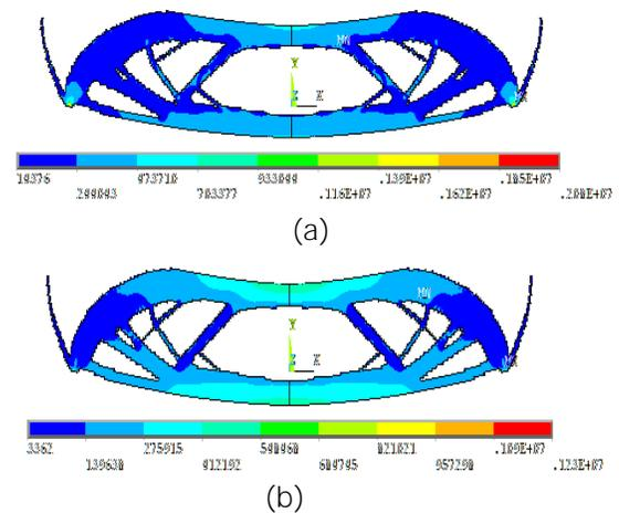
Fig. 1.4 Von mises stress induced in structure for (a) Isotropic (b) Orthotropic
