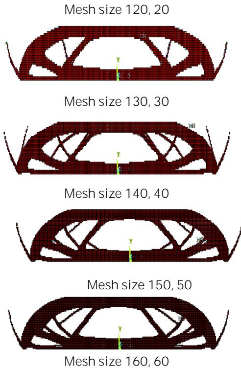
Fig. 3.1 Optimal topologies for different mesh densities for IM Model 5 ( $V_0 = 50\%$ )
