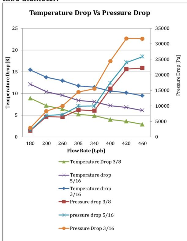
Figure no 3.3 Temperature drop & Pressure drop vs flow rate for various tube diameter.
