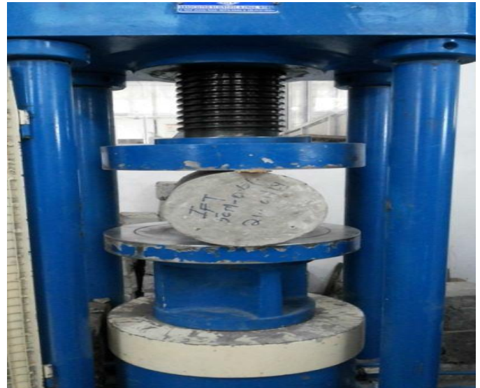
Fig -3: Tensile strength test on concrete cylinders
