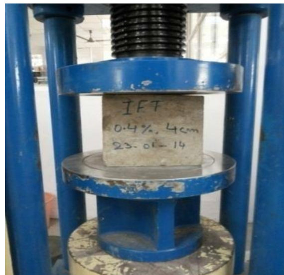
Fig -2: Compressive strength test on concrete cube
