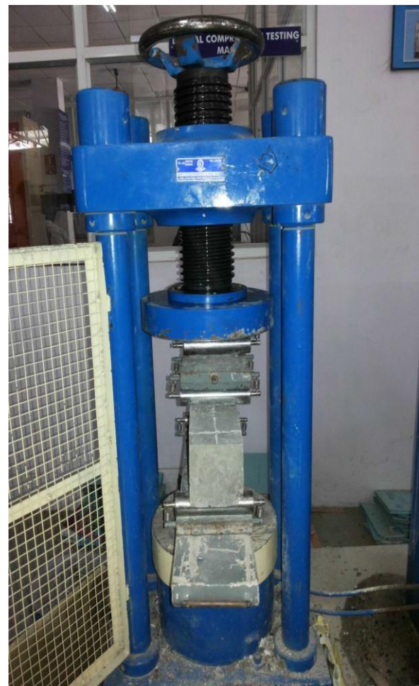
Fig -4: Flexure Strength test on concrete beam
