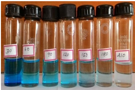
Fig.6. Gradual change in dye color from blue to colorless denotes dye degradation
