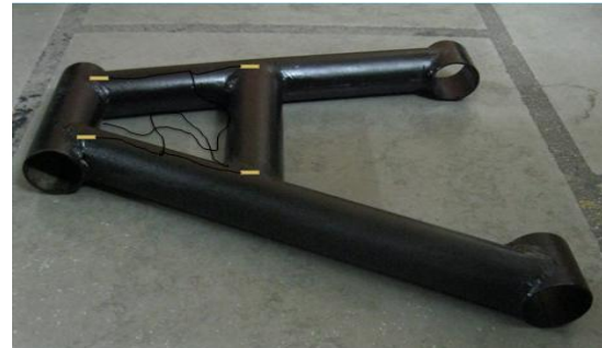
Fig.13. Actual Model of A - Type Suspension Arm with strain gauges.
