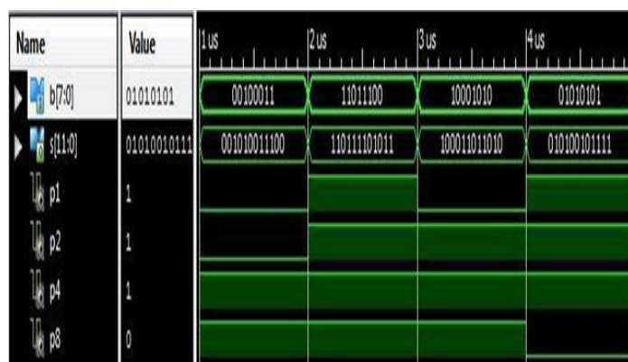
Fig. 4 Simulated Waveform of Encoder
