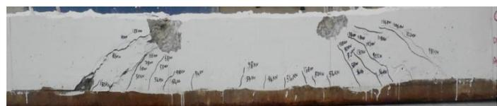
Fig-16: Typical failure pattern of composite beam specimen
