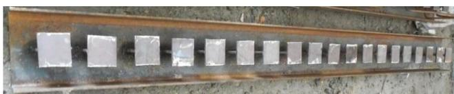
Fig-3: Type 1a shear connector welded to channel section
