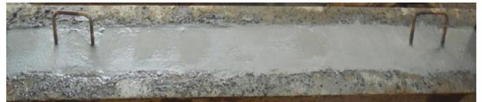
Fig-14: Beam specimen after casting
