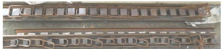
Fig-6: Type 2a Type 2b shear connector with stirrups welded to channel section
