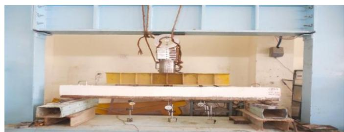
Fig-15: Beam specimen under testing
