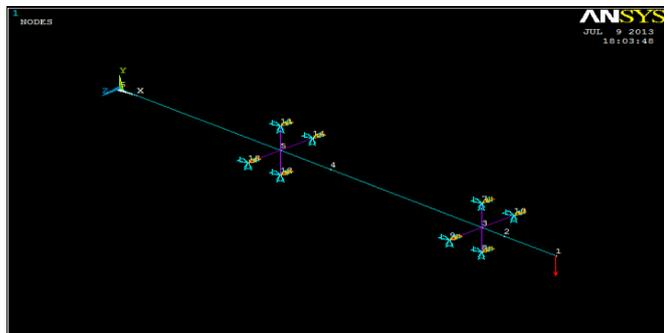
**Fig -7:** Finite element model of spindle with boundary conditions for static analysis
