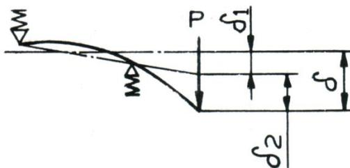
Fig -2: Spindle Deflection Diagram
