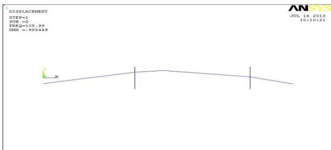
Fig -9: Mode shape at natural frequency 105.9Hz (Mode-2)
