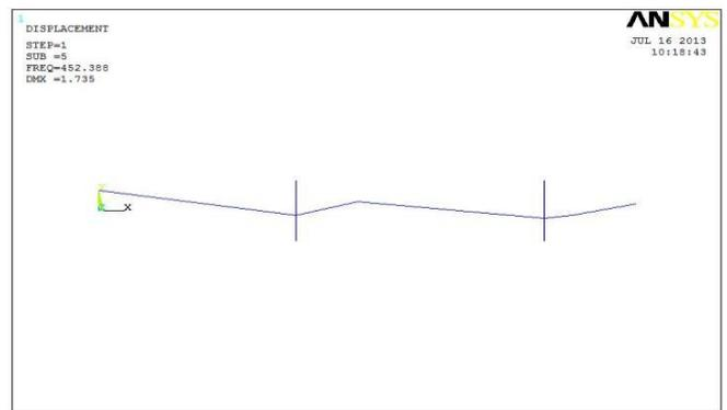
Fig -9: Mode shape at natural frequency 452.3Hz (Mode-5)
