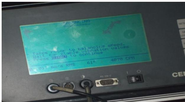
Fig -11: Vibration severity level of spindle on LCD
