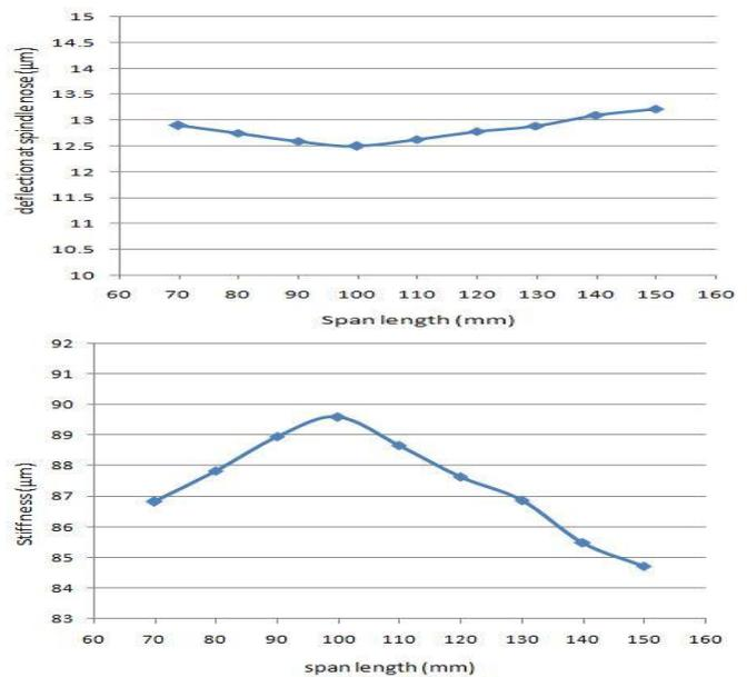
**Fig -3:** Variation of Spindle deflection and stiffness for different optimum span length
