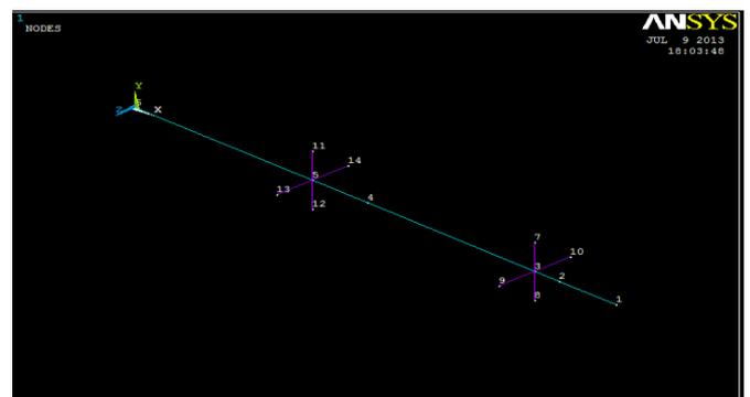
Fig -6: Finite element model of spindle for static deflection analysis
