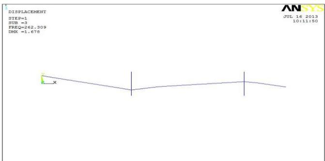
Fig -9: Mode shape at natural frequency 262.3Hz (Mode-3)
