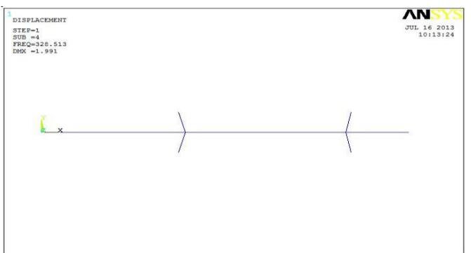
Fig -9: Mode shape at natural frequency 328.5Hz (Mode-4)
