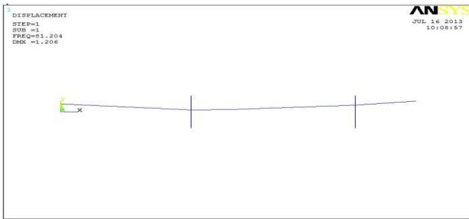
Fig -9: Mode shape at natural frequency 81.20Hz (Mode-1)
