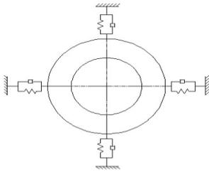
Fig -5: Layout of spring damper unit.
