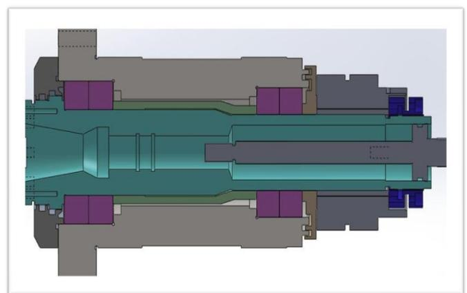
**Fig -1:** Typical spindle structure
