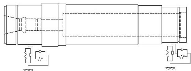
**Fig - 4:** Equivalent dynamic model of a spindle.
