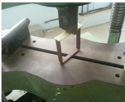
Fig-3: Mode II Interlaminar fracture toughness test
