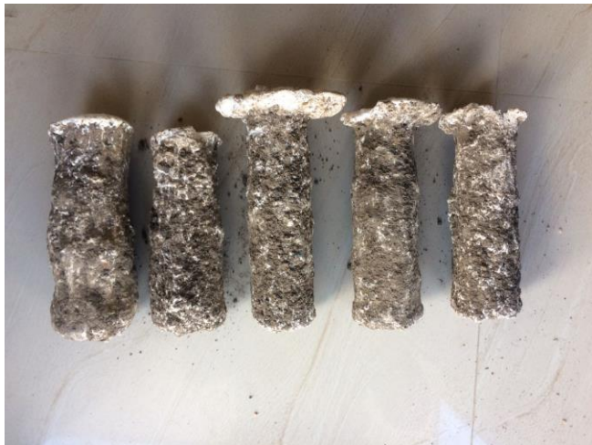
Fig 3.0 hardened models of reinforced stone columns with varying reinforcement depths at a spacing of D (5cm)
