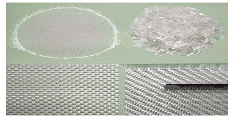
Figure1.3.3: Differences in the way the fibres are laid out give different strengths and ease of manufacture
