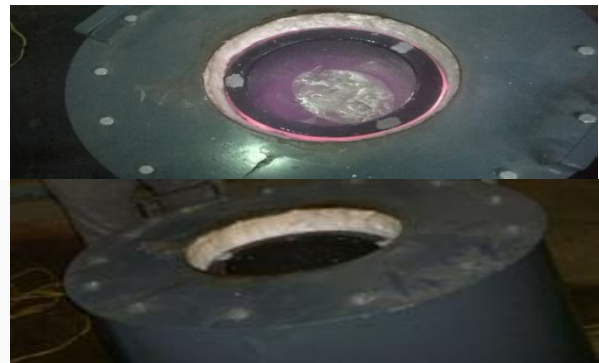
Figure1.4.8: Melting metal in a crucible for casting
