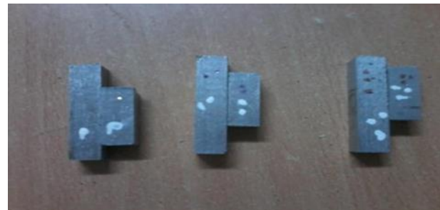
Fig-2: Impact testing specimens.
