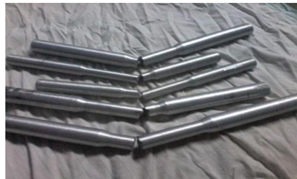
Fig-1: Tensile testing specimens.
