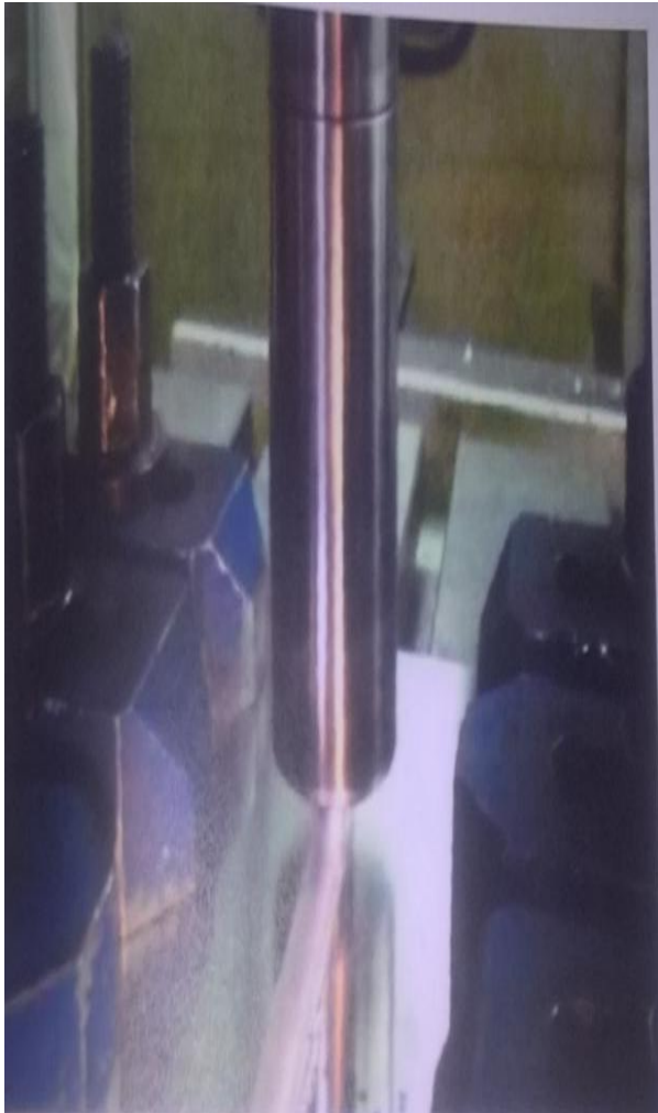
Fig-1: Friction stir welding process on AA5754 aluminium alloy
