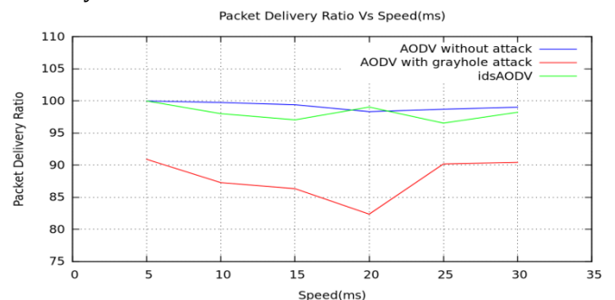
Figure 10: Packet Delivery Ratio vs. mobility for AODV
