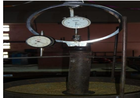
Fig 6: Mild steel footing and load connector
