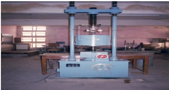
Figure 4: Static Loading Frame setup
