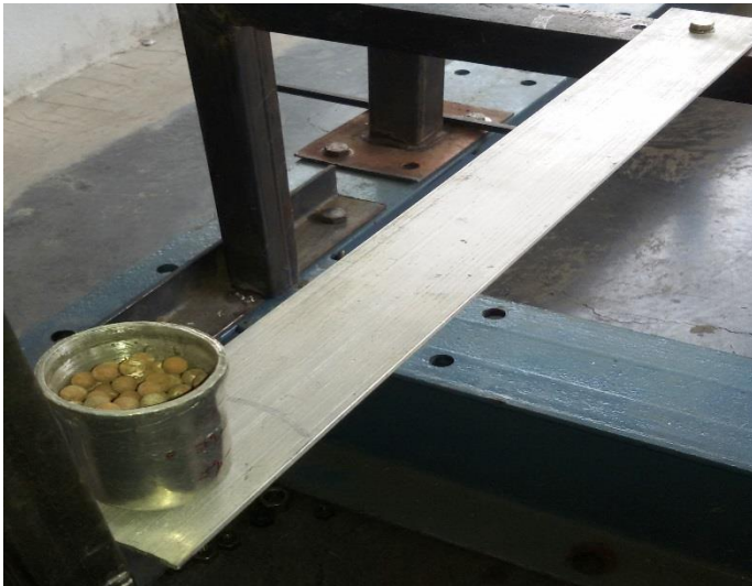
Fig 3:- Beam configured with particle impact damping
