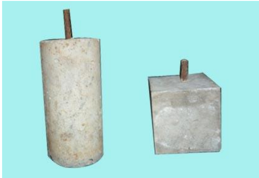
Fig. 3 Cylinder and cube specimen with the steel insertion
