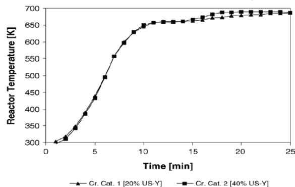
**Figure-2 Graph between temperature achieved and time of reaction**
