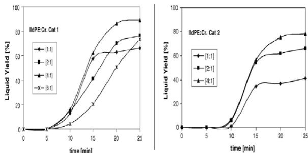
**Figure-3 Graph between liquid yield and time taken for various polymers to catalyst ratio**
