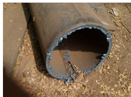
Figure E- Top view of MS pipe after being cut
