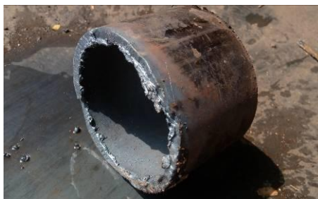
Figure F- Top view and side view of low carbon steel pipe post cutting
