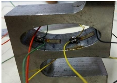
Fig -6: Strain gauge mounted on elliptical load cell
