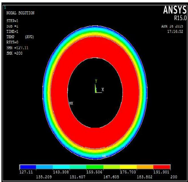
Fig.3- Temperature variation across the cylinder.
