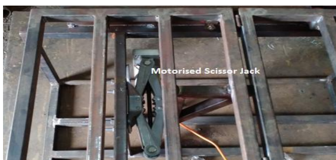
Fig -4 Motorised scissor jack attached at the back of wheelchair
