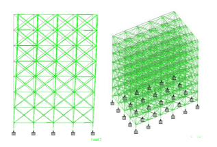
Fig.7:Deflected Shape of Frame with Infill wall Structure in Z- direction
