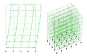
Fig.4: Deflected Shape of Bare Frame Structure in Zdirection
