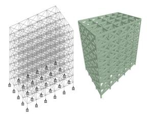
Fig.5: 3D View of G+6 Frame with Infill wall Structure
