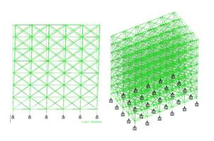
Fig.6: Deflected Shape of Frame with Infill wall Structure in X- direction
