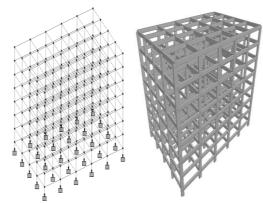
Fig.2: 3D View of G+6 Bare Frame Structure
