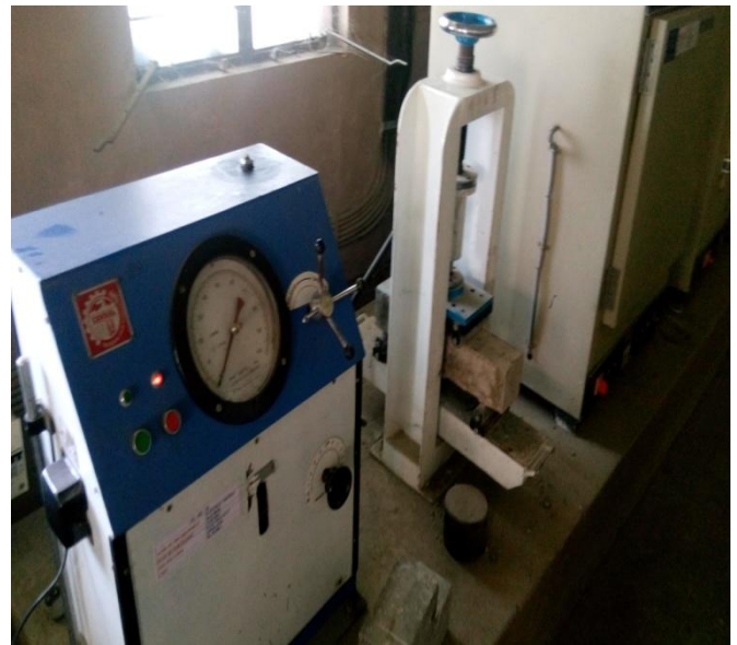
Fig -3: Flexural strength testing setup.
