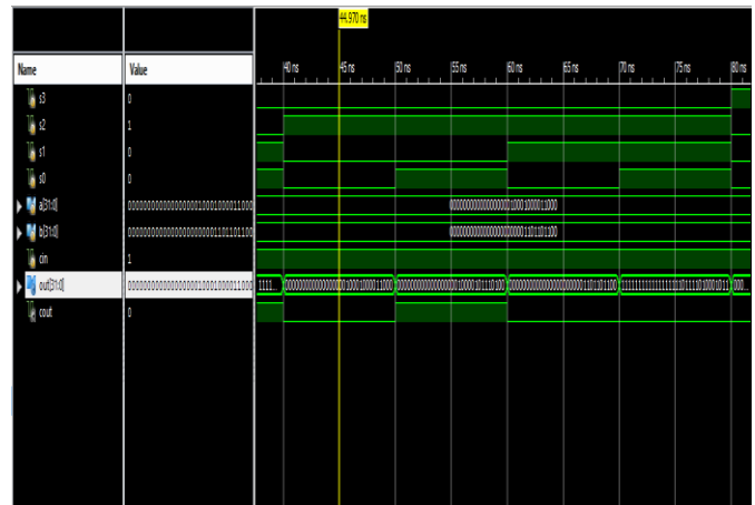
Figure 4.3: Result for 2 nd 4-operations (BUFFER A, EX-OR, BUFFER B and EX-NOR)
