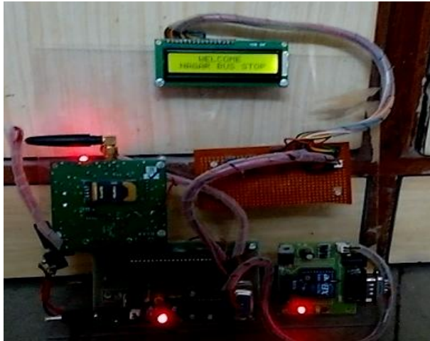
Fig -7: Bus Station Controller Module overview
