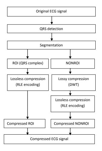
**Fig-1**: Compression of ECG signal
