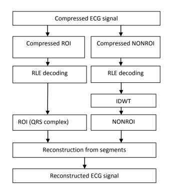
Fig- 2: Reconstruction of ECG signal
