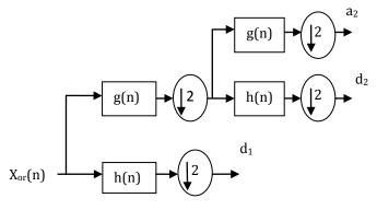
Fig - 4: Two level DWT decomposition.
