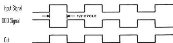
Fig. 5. Waveforms of JK flip-flop phase detector
