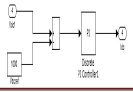
Fig-3 DC link voltage control using PI controller
