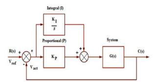
Fig-2Transfer function model of PI controller
