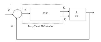
Fig-7 Block Diagram of Fuzzy Tuned PI Controller
