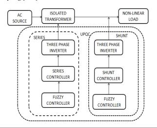
Fig-4 Block Diagram of Fuzzy Logic Controller
